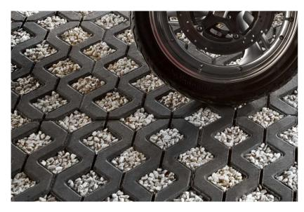
Hollow slabs are rectangular eco elements with characteristic incisions in the perimeter and holes inside the components. They are used primarily as the reinforcement of slopes, ditches, and the construction of parking garages and driveways. The holes are mostly often filled with grass or fine aggregate, which allows for the free movement of precipitation through the hollow slabs into the soil.
