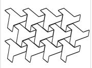
The sett with an regular edge line and flat surface. Spacers of classic size. The pattern consists of 1 element. The sett is made in double-filling technology. Joint width 3-5 mm.
